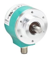
Lika Electronic AQ58 series incremental (quadrature) rotary encoder, medium duty, 5-30 VDC, radial exit, universal (line driver or NPN/PNP open collector) output, up to 14-bit (16384 ppr), 3/8in solid shaft, 58mm diameter body, IP65, M12 male.
