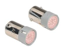
Fuji Electric bulb, LED, replacement, 24 VAC/VDC, BA9s/13 bayonet, red, 12 mA AC, 11 mA DC, 0.8W. Package of 2.
