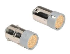
Fuji Electric bulb, LED, replacement, 24 VAC/VDC, BA9s/13 bayonet, orange, 12 mA AC, 11 mA DC, 0.8W. Package of 2.
