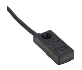
Koyo inductive proximity sensor, rectangular, 12 x 27 x 7mm body, polycarbonate housing, top sensing, NPN/PNP, N.O. output, 4mm sensing distance, non-flush, 200 Hz switching frequency, IP67, pigtail.
