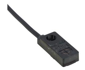
Koyo inductive proximity sensor, rectangular, 12 x 27 x 7mm body, polycarbonate housing, top sensing, NPN, N.C. output, 4mm sensing distance, non-flush, 200 Hz switching frequency, IP67, pigtail.
