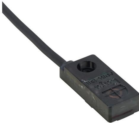
Koyo inductive proximity sensor, rectangular, 12 x 27 x 7mm body, polycarbonate housing, top sensing, NPN, N.C. output, 4mm sensing distance, non-flush, 200 Hz switching frequency, IP67, pigtail.
