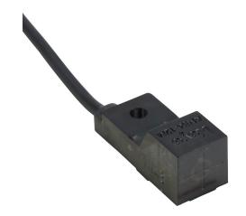
Koyo inductive proximity sensor, rectangular, 12 x 27 x 12mm body, polycarbonate housing, front sensing, NPN, N.C. output, 4mm sensing distance, non-flush, 200 Hz switching frequency, IP67, pigtail.
