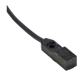
Koyo inductive proximity sensor, rectangular, 8 x 26.5 x 7.4mm body, polycarbonate housing, top sensing, NPN, N.O. output, 2.5mm sensing distance, non-flush, 500 Hz switching frequency, IP67, pigtail.
