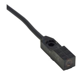
Koyo inductive proximity sensor, rectangular, 8 x 26.5 x 7.4mm body, polycarbonate housing, front sensing, NPN, N.O. output, 2.5mm sensing distance, non-flush, 500 Hz switching frequency, IP67, pigtail.
