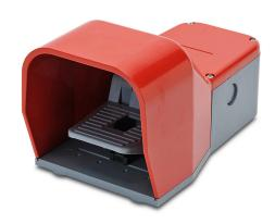
AutomationDirect electric foot switch, single, die-cast aluminum foot guard(s), red, maintained, (2) N.O. and (2) N.C. slow action contacts, ABS plastic operator, free moving pedal, gray, ABS plastic base.
