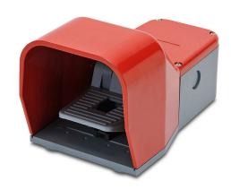
AutomationDirect electric foot switch, single, die-cast aluminum foot guard(s), red, maintained, (2) N.O. and (2) N.C. snap action contacts, ABS plastic operator, free moving pedal, gray, ABS plastic base.
