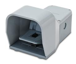
AutomationDirect electric foot switch, single, die-cast aluminum foot guard(s), gray, maintained, (2) N.O. and (2) N.C. snap action contacts, ABS plastic operator, free moving pedal, gray, ABS plastic base.
