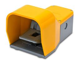
AutomationDirect electric foot switch, single, die-cast aluminum foot guard(s), yellow, maintained, (2) N.O. and (2) N.C. snap action contacts, ABS plastic operator, free moving pedal, gray, ABS plastic base.
