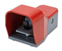
AutomationDirect electric foot switch, single, die-cast aluminum foot guard(s), red, momentary, (2) N.O. and (2) N.C. slow action contacts, ABS plastic operator, safety anti-trip pedal, gray, ABS plastic base.
