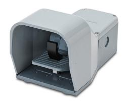
AutomationDirect electric foot switch, single, die-cast aluminum foot guard(s), gray, momentary, (2) N.O. and (2) N.C. slow action contacts, ABS plastic operator, safety anti-trip pedal, gray, ABS plastic base.
