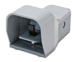
AutomationDirect electric foot switch, single, die-cast aluminum foot guard(s), gray, momentary, (2) N.O. and (2) N.C. snap action contacts, ABS plastic operator, safety anti-trip pedal, gray, ABS plastic base.
