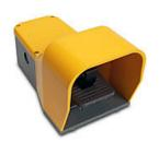
AutomationDirect electric foot switch, single, ABS plastic foot guard(s), yellow, momentary, (2) N.O. and (2) N.C. snap action contacts, ABS plastic operator, safety anti-trip pedal, gray, ABS plastic base.
