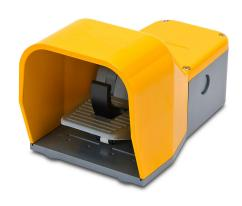
AutomationDirect electric foot switch, single, die-cast aluminum foot guard(s), yellow, momentary, (2) N.O. and (2) N.C. snap action contacts, ABS plastic operator, safety anti-trip pedal, gray, ABS plastic base.
