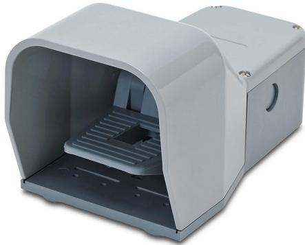
AutomationDirect electric foot switch, single, die-cast aluminum foot guard(s), gray, momentary, (2) N.O. and (2) N.C. slow action contacts, ABS plastic operator, free moving pedal, gray, ABS plastic base.
