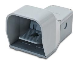
AutomationDirect electric foot switch, single, die-cast aluminum foot guard(s), gray, momentary, (2) N.O. and (2) N.C. snap action contacts, ABS plastic operator, free moving pedal, gray, ABS plastic base.
