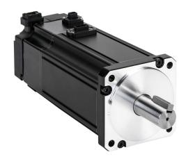
LS Electric low inertia AC brushless servo motor, 1 kW, 3-phase input, 17-bit (131072 ppr) encoder, integrated brake. For use with LS Electric L7C L7CA010U-AD 1 kW drive.
