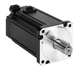
LS Electric low inertia AC brushless servo motor, 1 kW, 3-phase input, 17-bit (131072 ppr) encoder. For use with LS Electric L7C L7CA010U-AD 1 kW drive.
