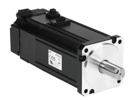
LS Electric low inertia AC brushless servo motor, 1 kW, 3-phase input, 19-bit (524288 ppr) encoder, integrated brake. For use with LS Electric L7PA010U-AD and iX7NHA010U-AD 1 kW drives and L7PA020U-AD and iX7NHA020U-AD 2 kW drives with 1-phase input.
