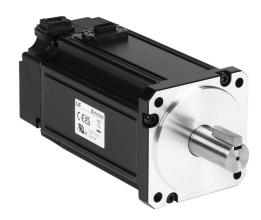
LS Electric low inertia AC brushless servo motor, 1 kW, 3-phase input, 19-bit (524288 ppr) encoder. For use with LS Electric L7PA010U-AD and iX7NHA010U-AD 1 kW drives and L7PA020U-AD and iX7NHA020U-AD 2 kW drives with 1-phase input.
