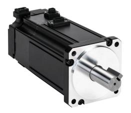
LS Electric low inertia AC brushless servo motor, 750W, 3-phase input, 17-bit (131072 ppr) encoder, integrated brake. For use with LS Electric L7C L7CA010U-AD 1 kW drive.
