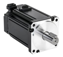
LS Electric low inertia AC brushless servo motor, 750W, 3-phase input, 17-bit (131072 ppr) encoder. For use with LS Electric L7C L7CA010U-AD 1 kW drive.
