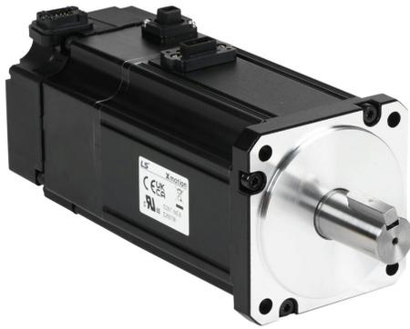
LS Electric low inertia AC brushless servo motor, 750W, 3-phase input, 19-bit (524288 ppr) encoder, integrated brake. For use with LS Electric L7PA010U-AD 1 kW drive and iX7NHA008U-AD 750W drives.
