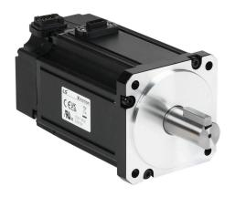
LS Electric low inertia AC brushless servo motor, 750W, 3-phase input, 19-bit (524288 ppr) encoder. For use with LS Electric L7PA010U-AD 1 kW drive and iX7NHA008U-AD 750W drives.
