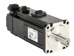
LS Electric low inertia DC brushless servo motor, 300W, 3-phase input, 19-bit (524288 ppr) encoder, integrated brake. For use with LS Electric PHOX-06-080NS-AD 6A drive.
