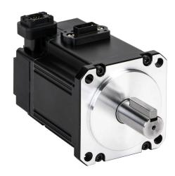
LS Electric low inertia AC brushless servo motor, 200W, 3-phase input, 17-bit (131072 ppr) encoder. For use with LS Electric L7C L7CA004U-AD 400W drive.
