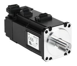
LS Electric low inertia AC brushless servo motor, 200W, 3-phase input, 19-bit (524288 ppr) encoder, integrated brake. For use with LS Electric L7PA004U-AD and iX7NHA004U-AD 400W drives.
