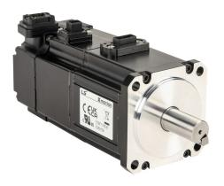
LS Electric low inertia DC brushless servo motor, 200W, 3-phase input, 19-bit (524288 ppr) encoder, integrated brake. For use with LS Electric PHOX-06-080NS-AD 6A drive.
