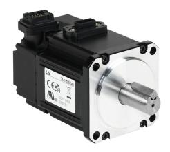
LS Electric low inertia AC brushless servo motor, 200W, 3-phase input, 19-bit (524288 ppr) encoder. For use with LS Electric L7PA004U-AD and iX7NHA004U-AD 400W drives.
