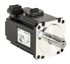
LS Electric low inertia DC brushless servo motor, 200W, 3-phase input, 19-bit (524288 ppr) encoder. For use with LS Electric PHOX-06-080NS-AD 6A drive.
