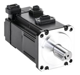
LS Electric low inertia AC brushless servo motor, 100W, 3-phase input, 17-bit (131072 ppr) encoder, integrated brake. For use with LS Electric L7C L7CA004U-AD 400W drive.
