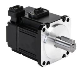
LS Electric low inertia AC brushless servo motor, 100W, 3-phase input, 17-bit (131072 ppr) encoder. For use with LS Electric L7C L7CA004U-AD 400W drive.
