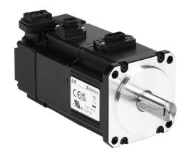
LS Electric low inertia AC brushless servo motor, 100W, 3-phase input, 19-bit (524288 ppr) encoder, integrated brake. For use with LS Electric L7PA004U-AD and iX7NHA004U-AD 400W drives.
