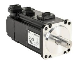
LS Electric low inertia DC brushless servo motor, 100W, 3-phase input, 19-bit (524288 ppr) encoder, integrated brake. For use with LS Electric PHOX-03-080NS-AD 3A drive.
