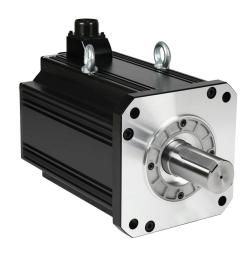
LS Electric medium inertia AC brushless servo motor, 7.5 kW, 3-phase input, 19-bit (524288 ppr) encoder. For use with LS Electric L7PB075U-AD 7.5 kW drive.
