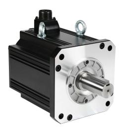
LS Electric medium inertia AC brushless servo motor, 5.5 kW, 3-phase input, 19-bit (524288 ppr) encoder. For use with LS Electric L7PB050U-AD 5 kW drive.
