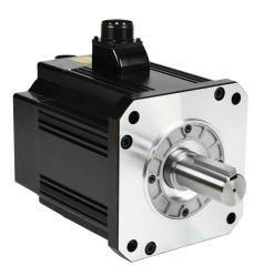
LS Electric medium inertia AC brushless servo motor, 3.5 kW, 3-phase input, 19-bit (524288 ppr) encoder, integrated brake. For use with LS Electric L7PB035U-AD 3.5 kW drive.
