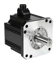
LS Electric medium inertia AC brushless servo motor, 3.5 kW, 3-phase input, 19-bit (524288 ppr) encoder. For use with LS Electric L7PB035U-AD 3.5 kW drive.
