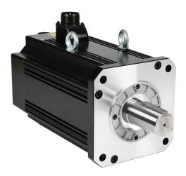
LS Electric medium inertia AC brushless servo motor, 7.5 kW, 3-phase input, 19-bit (524288 ppr) encoder, integrated brake. For use with LS Electric L7PA075U-AD 7.5 kW drive.
