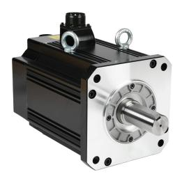
LS Electric medium inertia AC brushless servo motor, 5.5 kW, 3-phase input, 19-bit (524288 ppr) encoder, integrated brake. For use with LS Electric L7PA050U-AD 5 kW drive.
