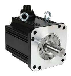
LS Electric medium inertia AC brushless servo motor, 5.5 kW, 3-phase input, 19-bit (524288 ppr) encoder. For use with LS Electric L7PA050U-AD 5 kW drive.
