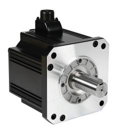
LS Electric medium inertia AC brushless servo motor, 3.5 kW, 3-phase input, 19-bit (524288 ppr) encoder. For use with LS Electric L7PA035U-AD and iX7NHA035U-AD 3.5 kW drives with 3-phase input.
