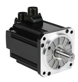
LS Electric medium inertia AC brushless servo motor, 2.2 kW, 3-phase input, 19-bit (524288 ppr) encoder. For use with LS Electric L7PB020U-AD 2 kW drive.
