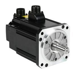
LS Electric medium inertia AC brushless servo motor, 1.6 kW, 3-phase input, 19-bit (524288 ppr) encoder, integrated brake. For use with LS Electric L7PB020U-AD 2 kW drive.
