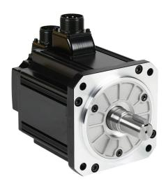
LS Electric medium inertia AC brushless servo motor, 1.6 kW, 3-phase input, 19-bit (524288 ppr) encoder. For use with LS Electric L7PB020U-AD 2 kW drive.
