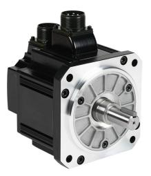
LS Electric low inertia AC brushless servo motor, 900W, 3-phase input, 19-bit (524288 ppr) encoder. For use with LS Electric L7PB010U-AD 1 kW drive.
