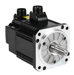
LS Electric low inertia AC brushless servo motor, 1.5 kW, 3-phase input, 19-bit (524288 ppr) encoder, integrated brake. For use with LS Electric L7PA020U-AD and iX7NHA020U-AD with 3-phase input and L7PA035U-AD and iX7NHA035U-AD with 1-phase input.
