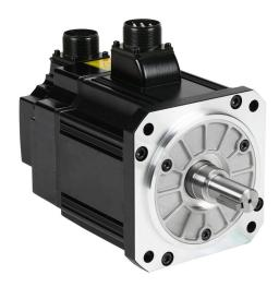
LS Electric low inertia AC brushless servo motor, 1.5 kW, 3-phase input, 19-bit (524288 ppr) encoder, integrated brake. For use with LS Electric L7PA020U-AD and iX7NHA020U-AD with 3-phase input and L7PA035U-AD and iX7NHA035U-AD with 1-phase input.
